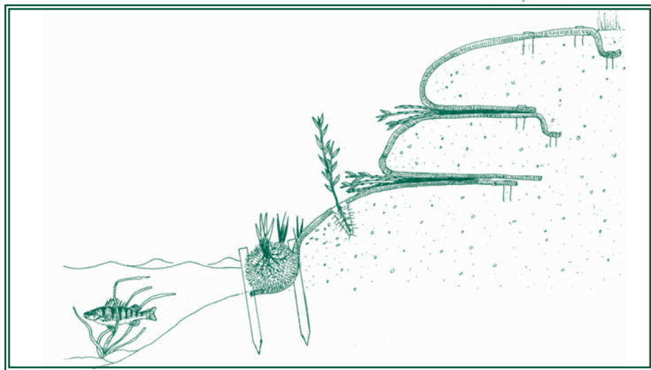
Typical Soil Bioengineering Cross-Section Using Coir Logs, Brush Layering, and Plants
